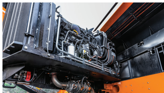
The entire engine unit swings out 90° from the machine for convenient maintenance access.
