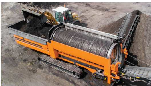
An optional 9.6 yd 3 hopper offers a low feed height and is driven by twin gear drives.
