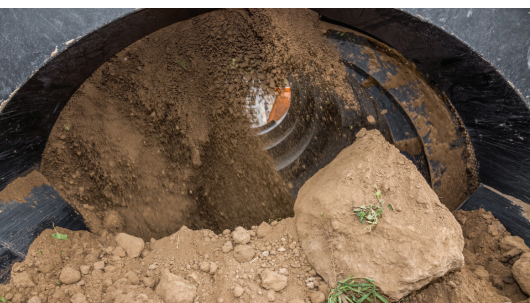
Auto load sensing varies the material flow from the hopper to consistently maintain peak output.
