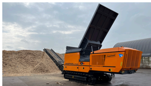
A hydraulically activated tipping hopper allows smart and efficient material feeding to the shaft.
