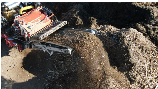
Wide belts and low bed depth so neodymium magnets can effectively remove metals.
