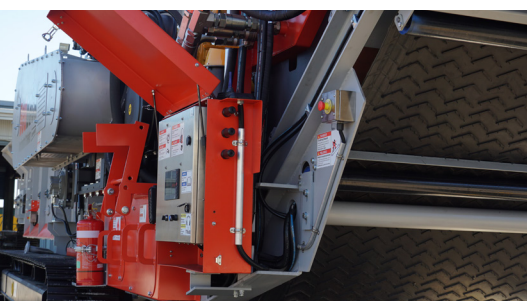
Contamination detection system disconnects drive when contamination is encountered
