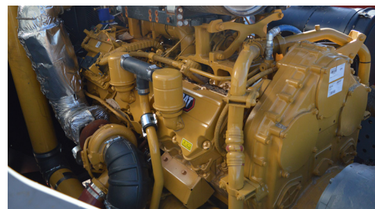
American-made Caterpillar diesel engine matched to a Twin Disc® for seamless control
