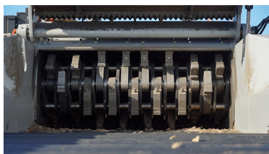
Rotor with adjustable hammers for multiple applications and easy onsite maintenance.
