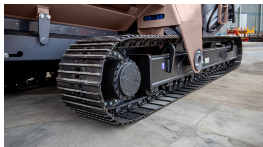
Heavy-duty steel tracks let you move and position the machine with ease—even in rough terrain.
