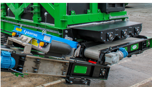
Auger discharge with variable water quench system driven by electric motor and gearbox.
