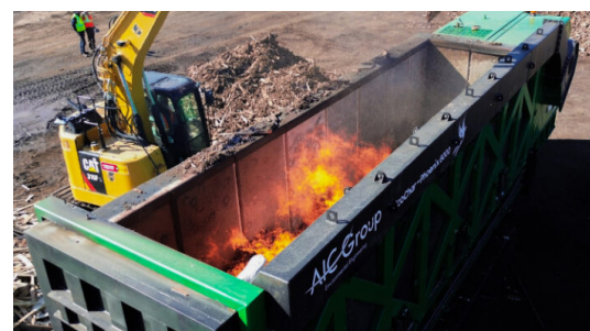
Refractory concrete panels and door rated to 3000° F.
