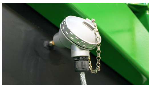
Temperature monitoring with 6 thermocouples rated to 3000° F.
