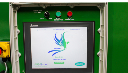
Intelligent Combustion Management System controls the process to ensure optimal operation and biochar production.
