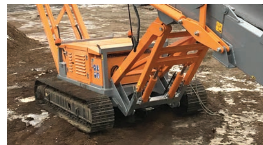
Heavy-duty tracks allow the conveyors to maneuver over rough and muddy terrain.
