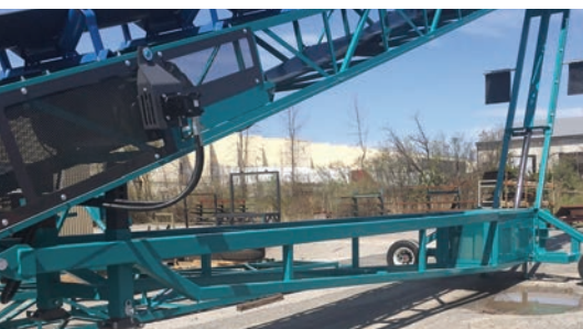
The hydraulic wrap drive provides maximum torque on the wheeled conveyors.
