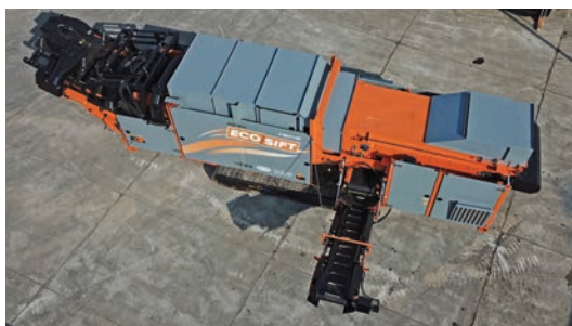
During settling in the expansion chamber, light fractions and foils are captured by the suction fans.
