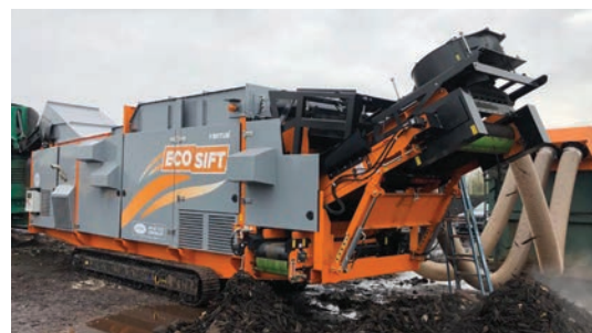
A powerful air knife blows light fractions and foils from the expansion chamber to the suction fans.
