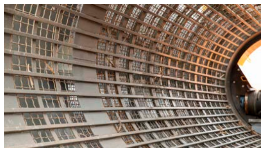
The heavy-duty inner drum can handle even the toughest overs, including rocks and debris.
