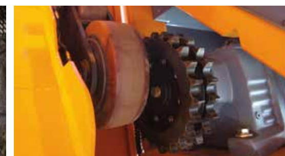
The trommel drum is driven by a double chain and sprocket that delivers exceptional torque.
