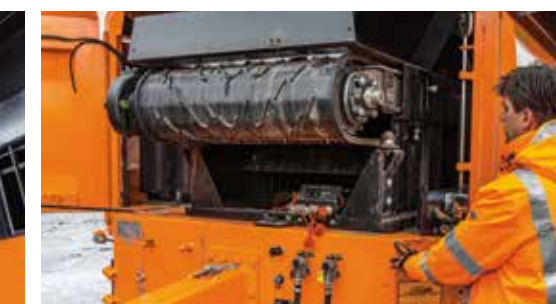
True modular construction allows easy access for operators and technicians.
