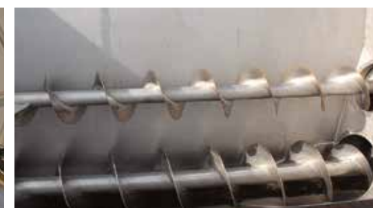
An auxiliary feed auger eliminates product bridging by reversing at programmable timed intervals.
