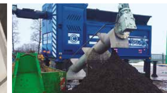
A high-speed vertical mill with bolt-on paddles extracts organics via centrifugal force.
