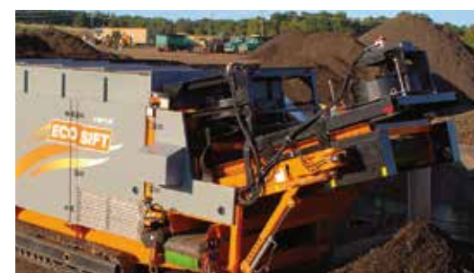
Any remaining contaminants are separated by dual suction fans, leaving a clean midsize fraction.
