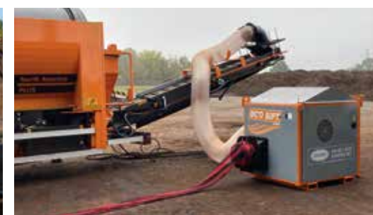
The hydraulically powered AERAS fits on any conveyor from 32" to 48" wide.
