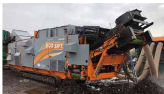
A powerful air knife blows light fractions and foils from the expansion chamber to the suction fans.
