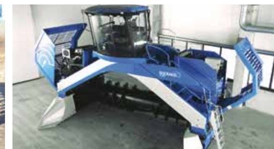
A fold-out work platform gives technicians clear access to the machine's components.
