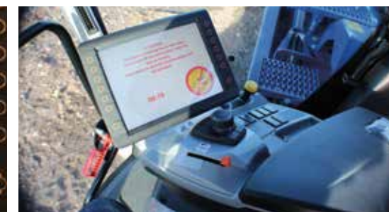
The single-joystick control, load-sensing and touchscreen display make for easy operation.
