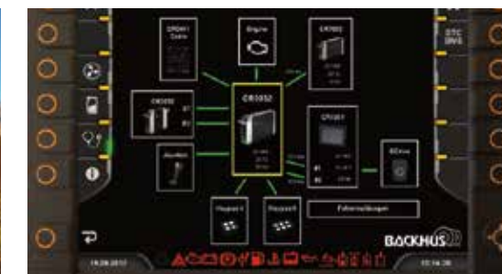
Self-diagnostic CAN bus system provides real-time feedback and alarms displayed in text format.
