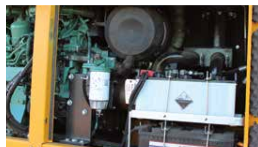
The rear-mounted engine compartment is fully accessible without the need for ladders or steps.
