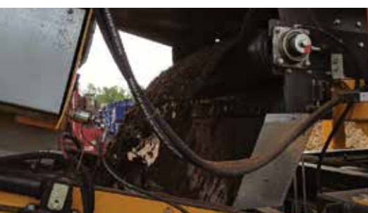
Hydraulic deck slider allows easy change from three-product to two-product configuration.
