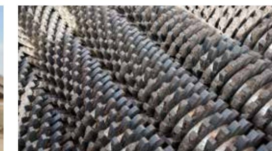
A four-bolt system connects the shaft and stars, creating stability and improving shaft tolerance.
