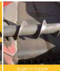
auger in hopper
