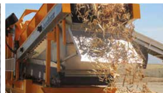
On three-fraction units, oversize material is only screened on the coarse deck to minimize wear.
